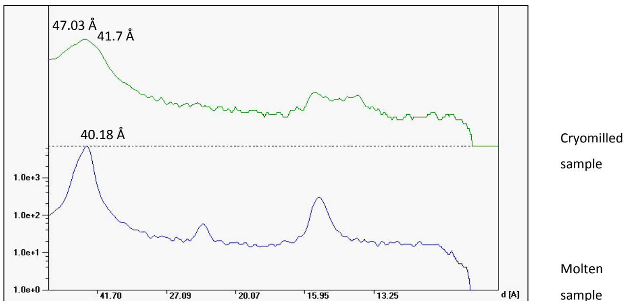
Figure 38. SAXS spectra of cryomilled Dynasan® 116/10% Tween® 65 in comparison to molten sample containing 10% Tween® 65.
