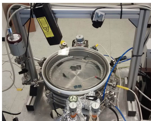
Figure 6.1: iCVD reactor that was used to synthesize MAA-PFDA polymers
