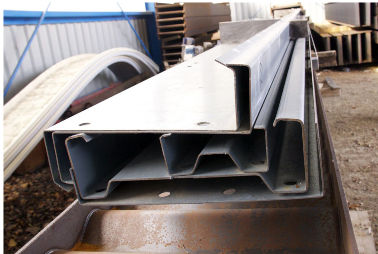
Figure 1.1: Photo of purlins.
