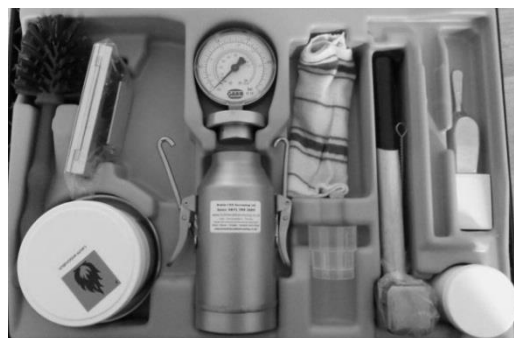
Abb. 65 Calciumcarbid Drucktestset (Mobile CAD Surveying, 2015)
