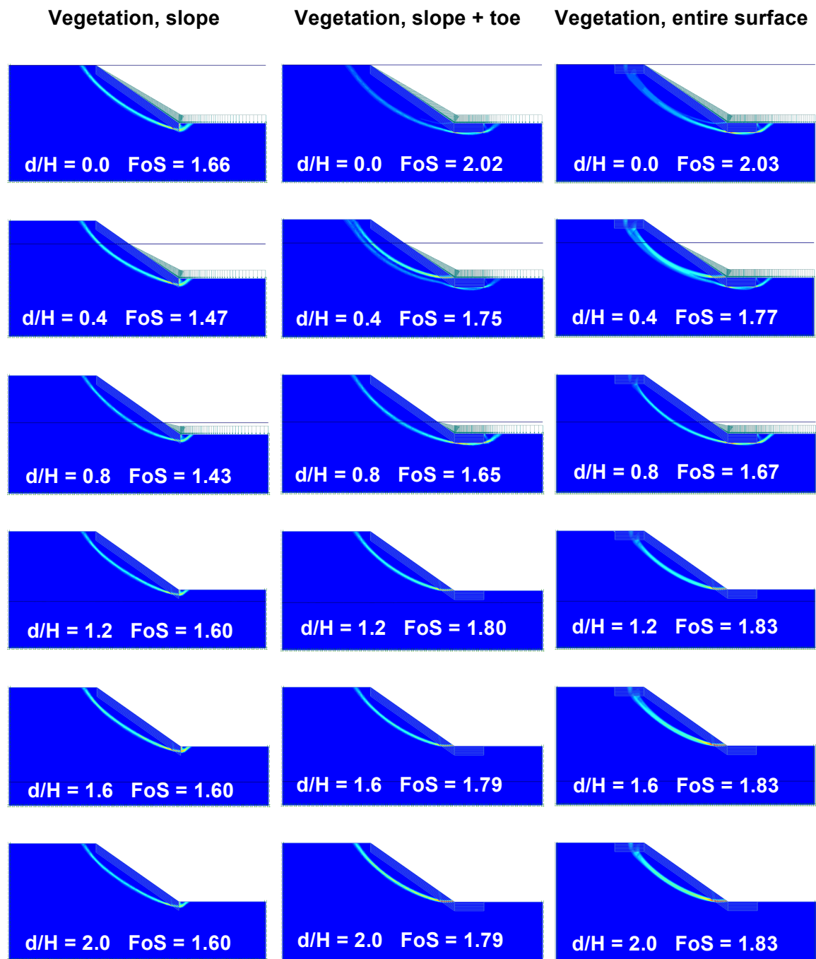
Fig. 41 Failure mechanism (incremental deviatoric strain) for soil 1, inclination 35 degree, left column vegetated slope, middle column slope + toe, right column entire surface vegetated
