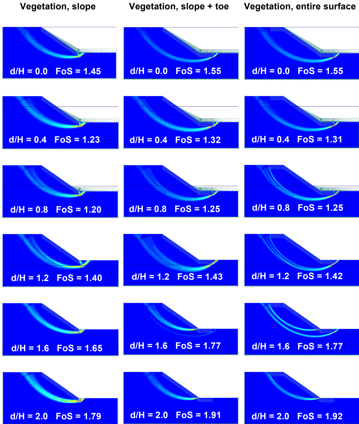
Fig. 42 Failure mechanism (incremental deviatoric strain) for soil 2, inclination 35 degree, left column vegetated slope, middle column slope + toe, right column entire surface vegetated
