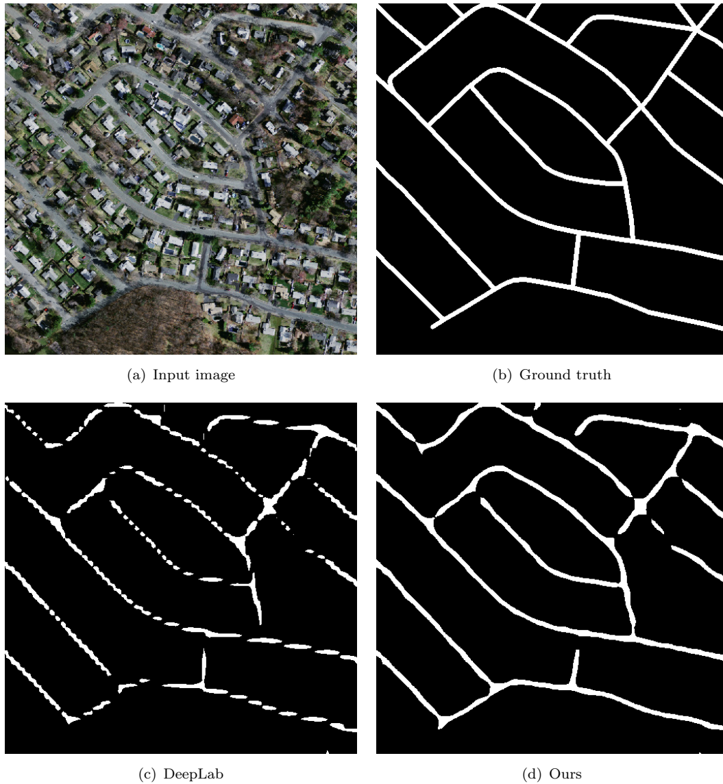
FIGURE 3.4: The images illustrate the segmentation results using the DeepLab-LargeFOV network and our proposed architecture. Figure 3.4(a) and 3.4(b) show the input image and the ground truth annotation. Figure 3.4(c) shows the aliased results using the DeepLab architecture and figure 3.4(d) shows our approach with the improved detection accuracy at small-scaled objects.
