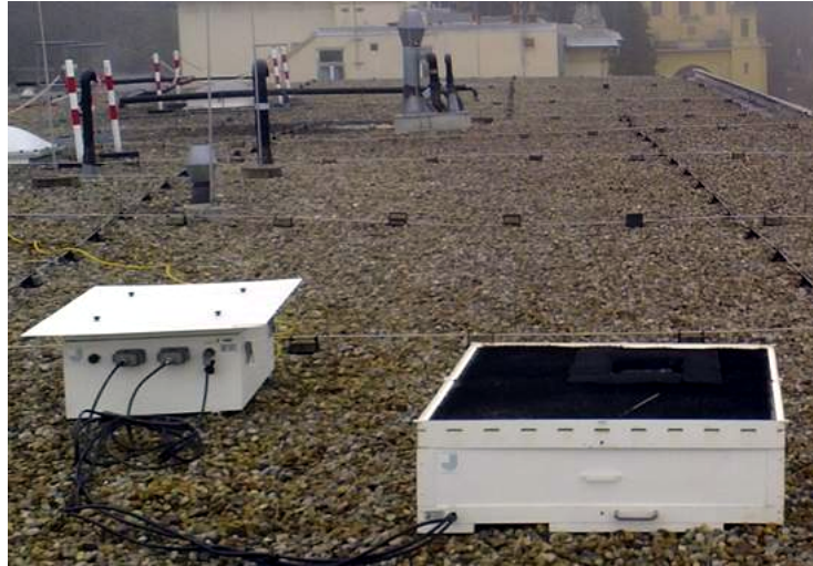
Figure 10: Sample Low Profile 2DVD setup
