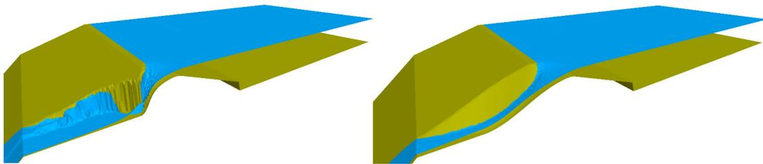
The breaching process without slide effect creates a very narrow and unnatural channel with steep side banks. On the other hand, the simulation with slide effect produces a much more realistic breach channel. Of course, the profiles of the channel axis fit much better with sediment slide.
