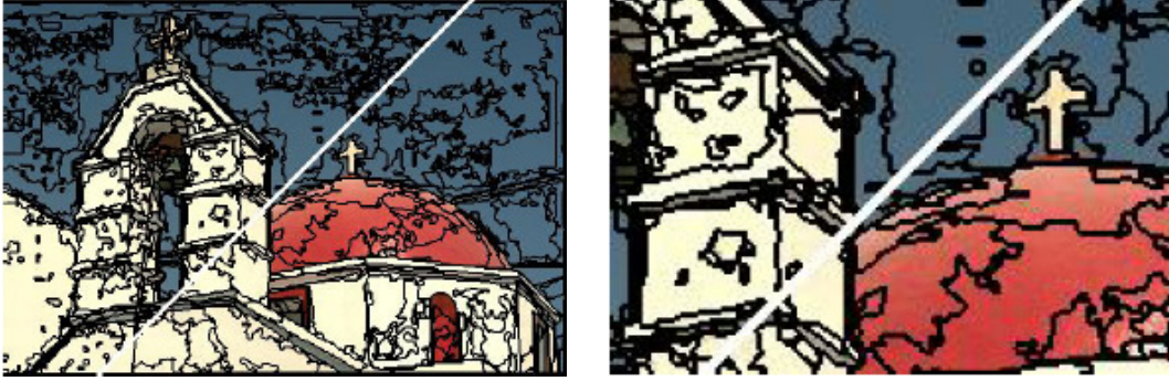
Figure 5.10: Visualization of superpixels generated by the algorithm of Felzenszwalb and Huttenlocher [19] with two different zoom-levels. Image courtesy of [1].
