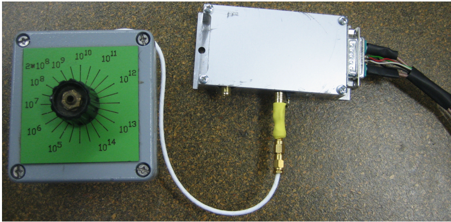
Figure 3.11.: Calibrating the Ion Probe electronics with a decade resistor. An adapter is needed to connect the coaxial SMC plug to the electronics' triaxial connector.
