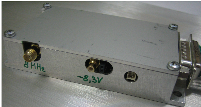
Figure 7.2.: Interface of an Analog Box. From the left: Cap Probe (SMA connector), Ion Probe (SMC connector + 2 pin header for outer triax shield), 2 pin connector for boom deployment microswitch, 7W2 connector to Main Box
