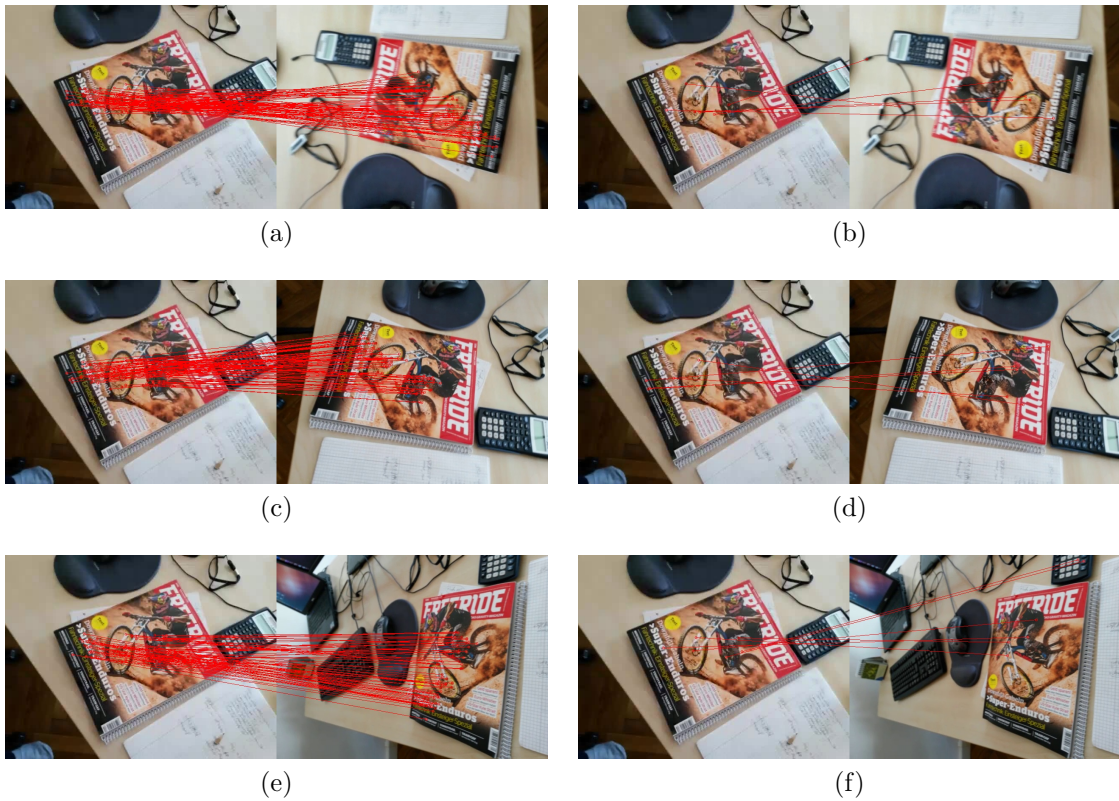
Figure 36: Detected interest points for individual frames and the correspondences to the model frame shown as red lines. The model image is on the left side. (a), (c), and (e) show the matches using the Direct Ordinal Ferns, and (b), (d), and (f) show the matches for the original RFe. Both methods use S = 7 features per fern and M = 20 ferns.
