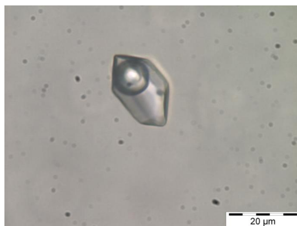
Fig.85: Three-phase FIA V3 consisting of H_2O liquid, CO_2 liquid, and CO_2 vapour at room temperature. This inclusion represents a primary characteristic.
