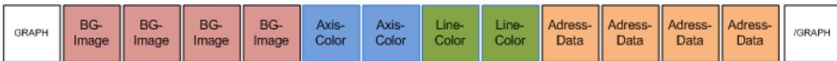
Figure 6.12: A diagram of the structure of the Graph -component in bytecode. It can be used to tackle the task of presenting large amounts of data in an intuitive, visually appealing way. The first four bytes that are parsed hold the address of an image that is used as a background that fills the entire component. The next two words contain first the pen-color that is used to draw the chart's axis and that of the plotted line that represents the data. Finally, in the last 4 bytes, the address that points to the data on the SD-card is encoded.
