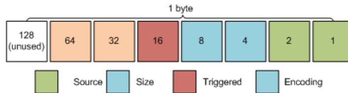
Figure 6.5: Apart from some attributes that are always encoded directly into the bytecode, such as the dimensions of a Tile , whenever an attribute is parsed its property header is read. This one-byte space within the bytecode contains a number of flags upon which the interpreter determines an attribute's size, source, encoding and if the attribute contains a Trigger .
