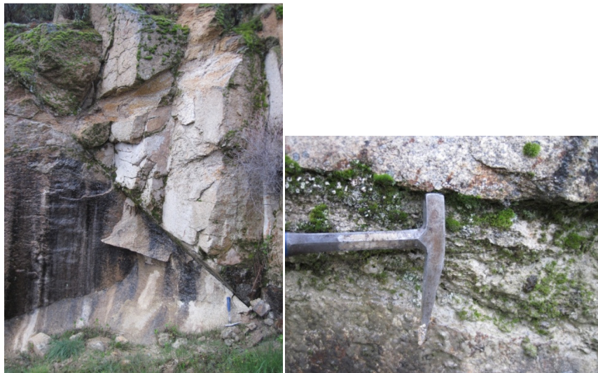
Figure 6.23 – Typical weathering situation close to the surface and along discontinuity plane
