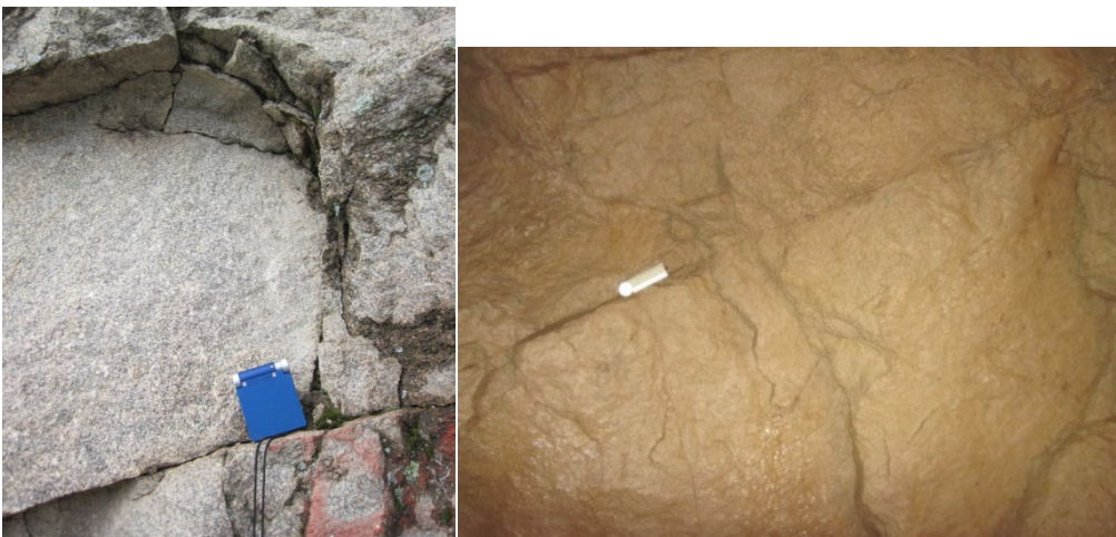
Figure 6.25 – Typical joint plane apertures at the surface and underground
