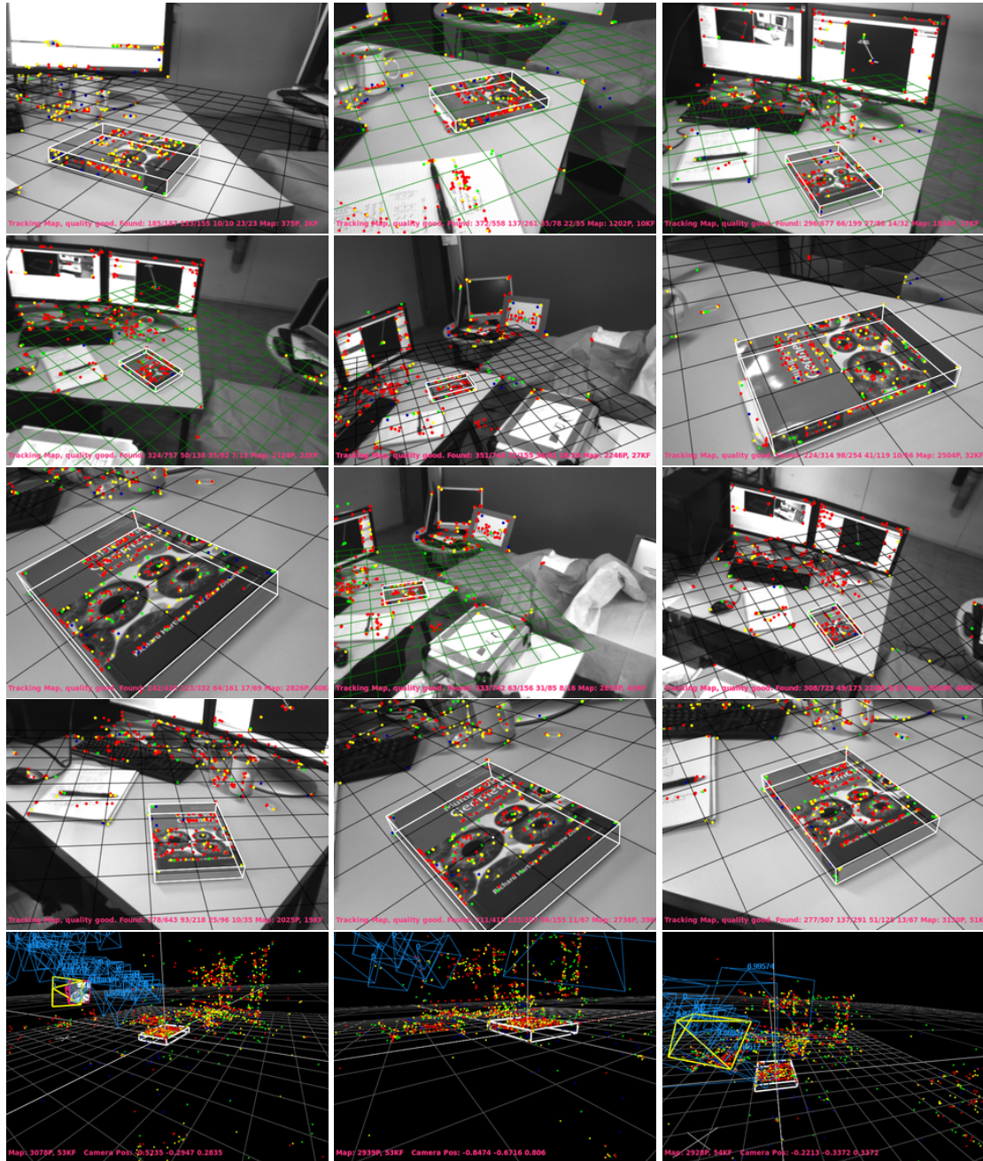
Figure 5.9: A few qualitative results of our implementation are shown here. The high accuracy is visible, especially when being close to the object. Obtaining such highly accurate results is only possible when the initialization is excellent, which is assured by refining the first and second keyframe during initialization. The bottom row shows the final map.
