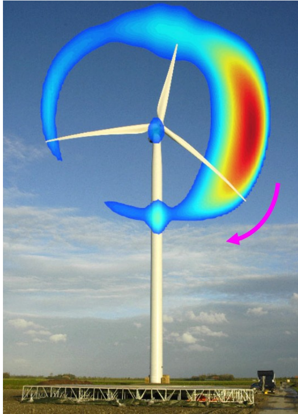
Figure 1.5.: Wind turbine noise source distribution in the rotor plane of a GE 2.3MW prototype test turbine. Rotor diameter 94m, tower height 100m. [27, 28]
