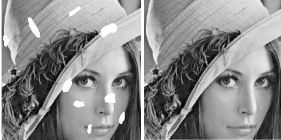
Figure 1.3: Inpainting result using variational inpainting. The corrupted parts of the original image have been completely removed and the result looks very natural. [Images taken from [Mas02]]
