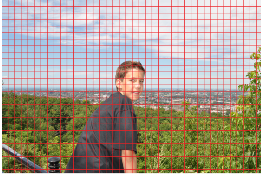
Figure 3.4: This Figure illustrates a CUDA computing grid for an example image ( 640 \times 480 ). The red lines define the borders of the blocks ( 16 \times 16 ). Note that it is usually not possible to define in what order the blocks are being executed.
