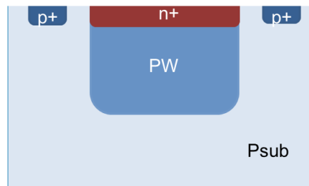
Figure 23: Schematic structure of photodiode with a n^+ -well in p-well in lightly p-doped substrate. The meaning of the labels of the structures is explained in Table 2
