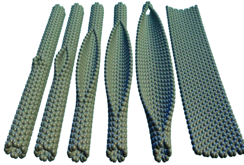
Figure 2.2: Schematic outline of the longitudinal unzipping of a CNT to form a GNR (adapted from Ref. [8]).
