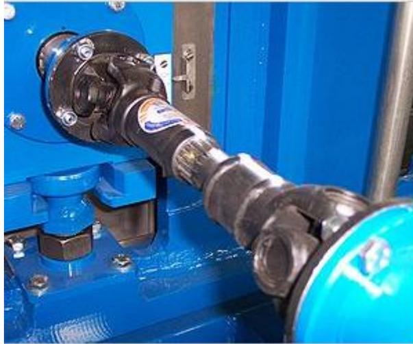
**Figure 9.** Drive shaft<sup>1</sup> with universal joint at each end and a spline in the centre [14].
