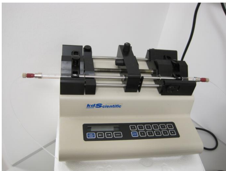
Fig. 35: Injecting/withdrawing syringe pump (KDS-260-CE, kdScientific, USA).
