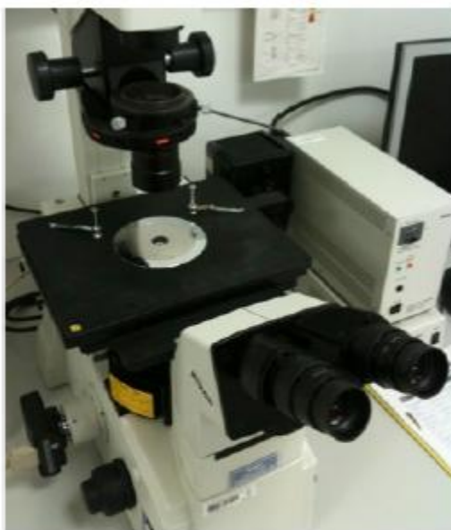
Fig. 27: Eclipse TE2000-S inverted fluorescence microscope (Nikon Instruments, Japan).
