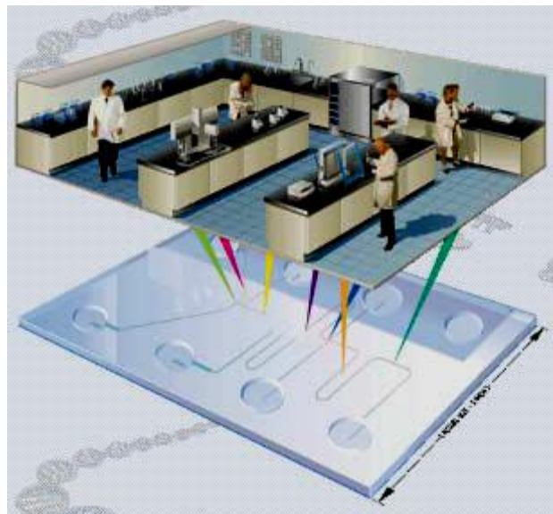
Fig. 9: Schematic of how laboratory functions are confined in a microchip (37).
