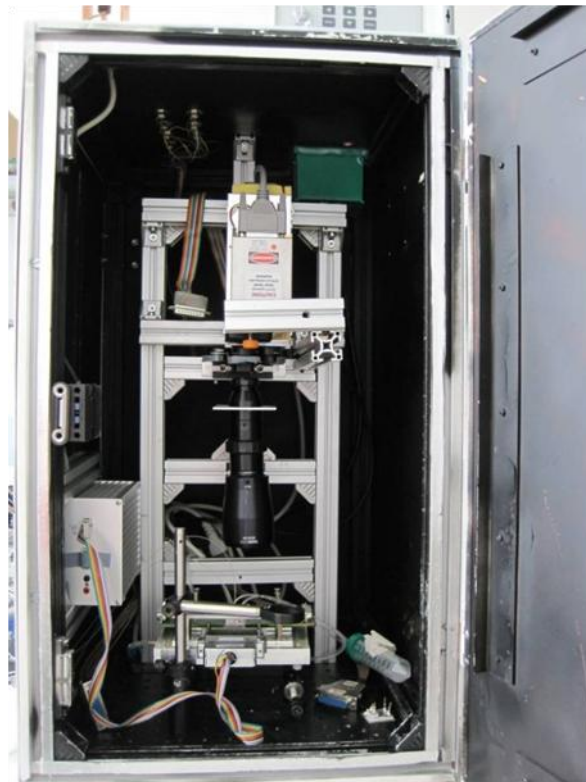
Fig. 39: Siemens-Box consisting of light source, neutral density filter, aperture, microchip mounting station, notch filter and OPDs.
