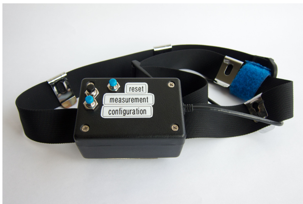
Figure 3.9: The figure shows the black case which includes the sensorplatform Neon, the GPS module and the battery. The three buttons are for the three possible modes configuration, measurement and reset.
