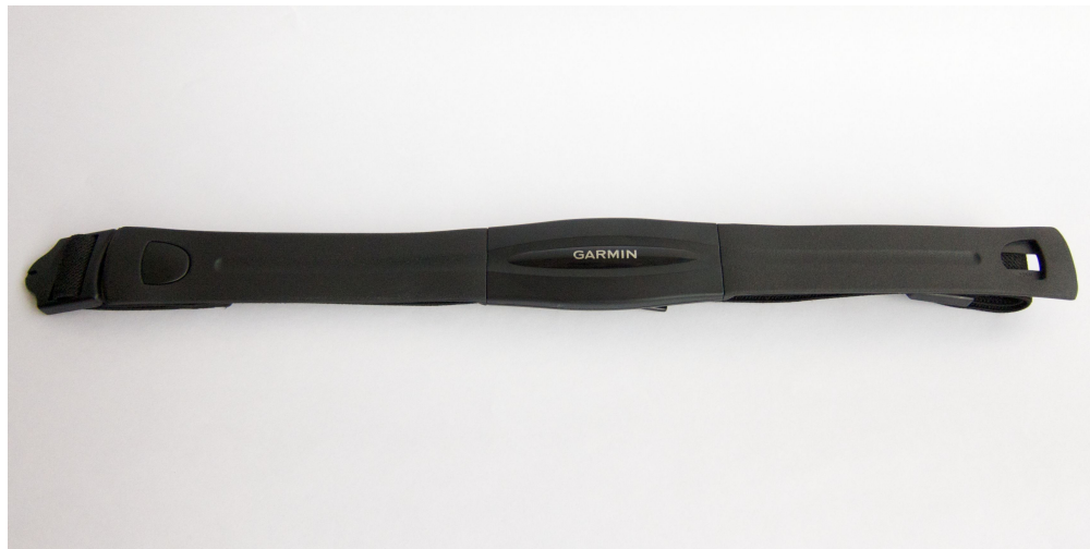
Figure 3.6: Garmin chest strap to determine the heart rate of the subject.
