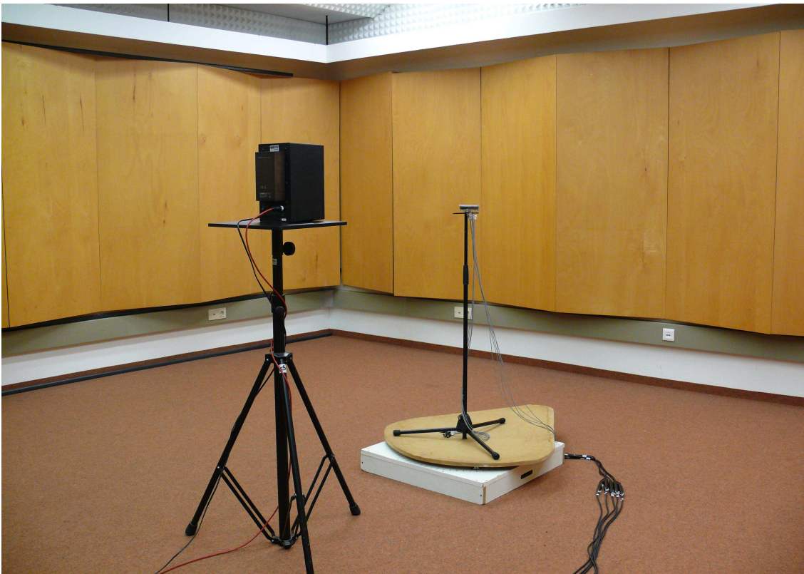
Figure 5.5: Recording setup for the beam pattern measurement in the recording studio (SPSC Lab).
