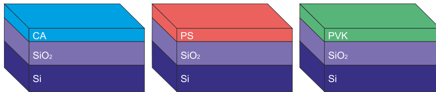
Figure 4.1.: CA, PS and PVK single layers on thermally oxidized silicon substrates.
