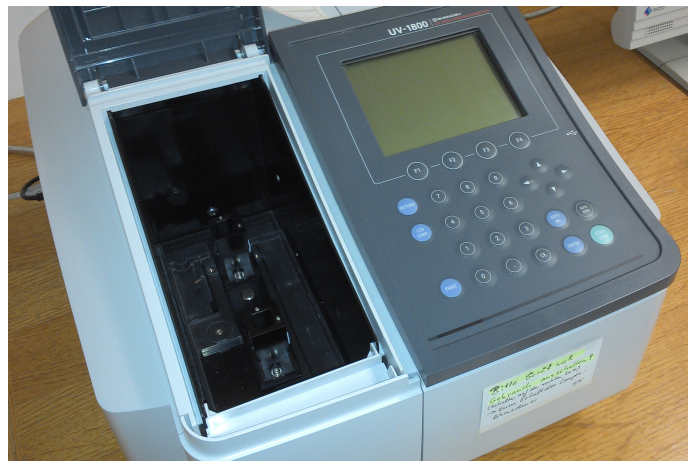
Figure 3.14.: Sample chamber of the UV-1800 from Shimadzu .
