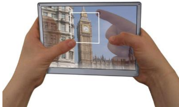
Figure 8: Concept sketch of LucidTouch: a pseudotransparent device (Wigdor et al., 2007)
