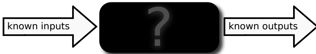
Figure 1.3: Black-Box testing scheme
