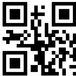
Figure 2.4: Example for an artificial landmark. QR tag with encoded text "kitchen".
