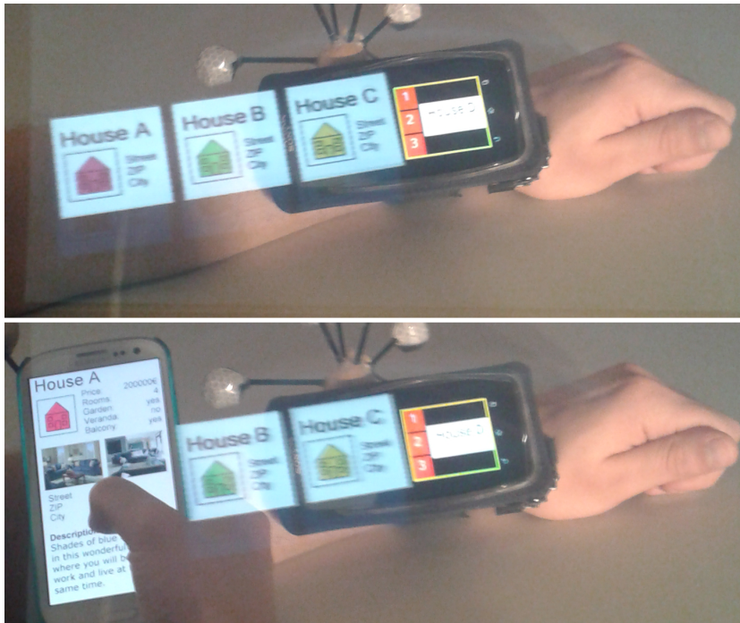
Figure 5: Arm clipboard with preview icons laid out on arm (top). Spatial pointing enables switching to high fidelity on a smartphone (bottom).
