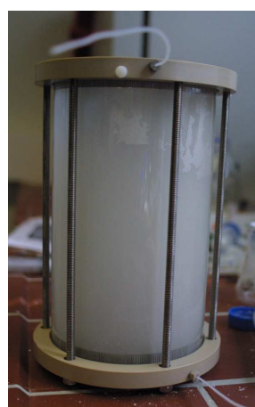
Figure 1. left: Annular filling frame; right: Scheme of an annular chromatographic operation. [10]
