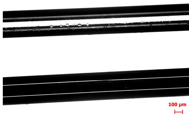
Figure 17. 50 times magnified picture of an empty (top) and filled (bottom) capillary.
