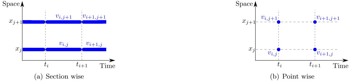
Figure 5.11: Difference between section-wise and point-wise defined spatio-temporal data. Section-wise data is defined over a spatio-temporal region as shown in (a), whereas point-wise data is solely defined on points as shown in (b)
