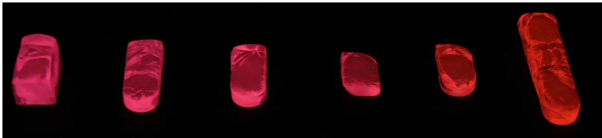
Figure 29: Glass samples with the composition 10-90-0 AD1000 prepared with different melting times, photographed under UV light with a wavelength of 365 nm. Melting times were, from left to right: 30 min, 1h, 1 h 15 min, 1 h 30 min, 1 h 45 min and 2 h.
