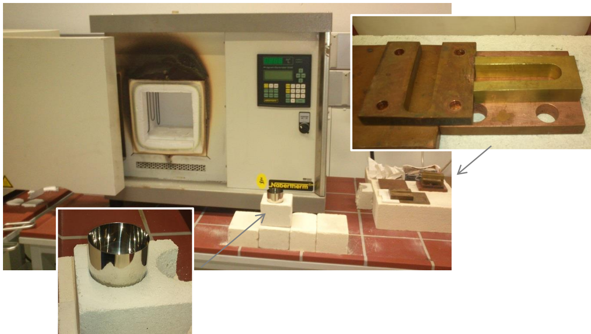
Figure 13: Picture of the oven with magnifications of the crucible and the copper mould.
