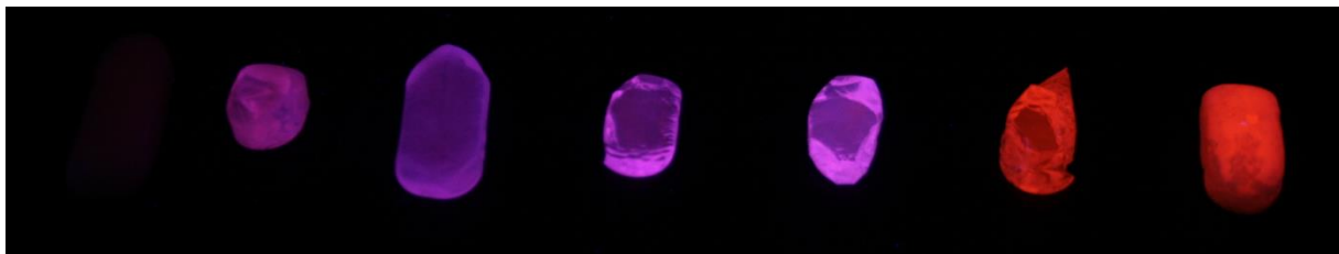
Figure 35: Glass samples with different amount of Na 2 O, melted at 1000 °C* for 1 h and quenched on air with no further heat treatment, photographed under UV light at a wavelength of 365 nm. The compositions were, from left to right: 0-100-0, 5-95-0, 10-90-0, 15-85-0, 20-80-0, 30-70-0 and 45-55-0. *0-100-0: after 1 h increase to 1200°C for 1 h.
