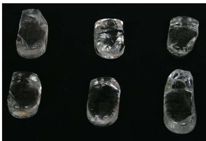
Figure 42: Glass samples with the following compositions, melted at 1300 °C for 1 h and quenched on air with no further heat treatment, were photographed in daylight. Top - from left to right: 9.5-85.5-5, 9.4-84.6-6 and 9-81-10. Bottom - from left to right: 10-85-5, 9-85-6 and 5-85-10.
