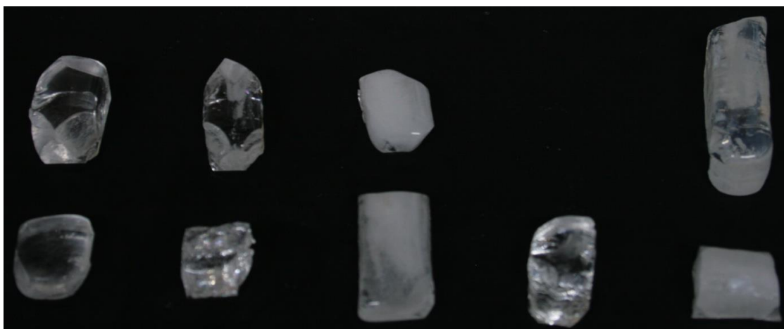
Figure 38: Glass samples photographed in daylight. Top - from left to right: 10-90-0 AD1000 2 h, 9-81-10 AD1000 2 h, 8.5-76.5-15 AD1200 2 h and 8-72-20 AD1400 1 h 30 min. Bottom - from left to right: 10-90-0 AD1000 1 h, 9-81-10 AD1000 1 h, 8.5-76.5-15 AD1200 1 h, 8.5-76.5-15 AD1400 1 h and 8-72-20 AD1400 1 h.
