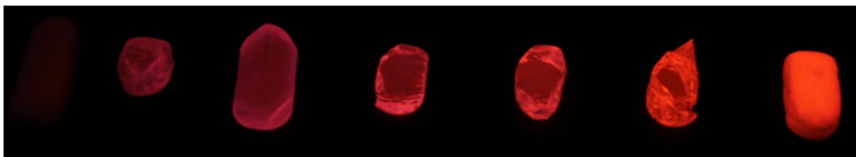
Figure 36: Glass samples with different amount of Na 2 O, melted at 1000 °C* for 1 h and quenched on air with no further heat treatment, photographed under UV light at a wavelength of 254 nm. The compositions were, from left to right: 0-100-0, 5-95-0, 10-90-0, 15-85-0, 20-80-0, 30-70-0 and 45-55-0. *0-100-0: after 1 h increase to 1200°C for 1 h.
