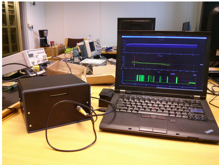
Figure 1.3.: Second iteration of the Project attached to a laptop with the visualisation. Behind the slit the sensor is placed. For test purposes the trigger is here connected to a signal generator.
