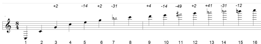
Figure 2.7: The natural harmonic scale for the key C3 (GNS: c ). The lower numbers indicate the number of the harmonic. The upper numbers become relevant in section 4.3.2. They indicate the deviation of the noted pitch and the frequency of the natural harmonic. The unit is cents.
