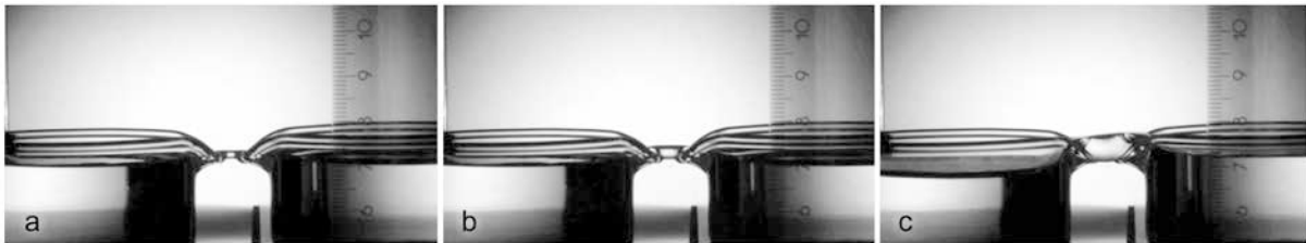
Fig. 11: Bridge diameter as function of applied potential and current in water (a: 7 kV, 5 mA; b: 11 kV, 5 mA; c: 22 kV, 5 mA)
