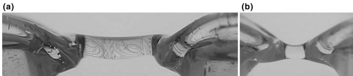
Fig. 7 a Horizontal liquid bridge in glycerol formed between two beakers, 16 kV DC. Polyamide tracers were added for stream line visualization, the picture is a 30 frames average. b Horizontal bridge formed at 15 kV AC, 11.5 kHz. No tracer movement can be observed
