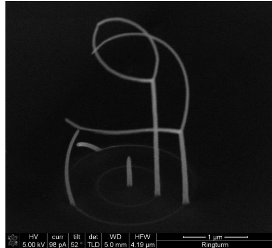
Figure 69: lassos with radii 500 nm and 1 μm respectively. Fabricated with pillar bow strategies and single pillar (center).
