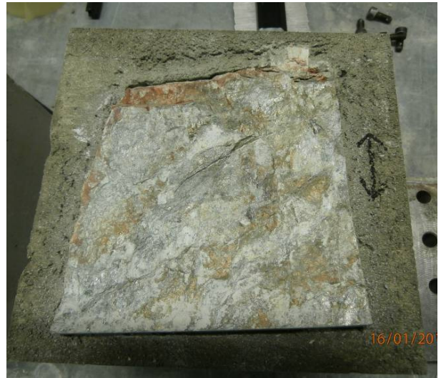
Sample half of the lower shear box after shearing (arrow marks the shear direction)
