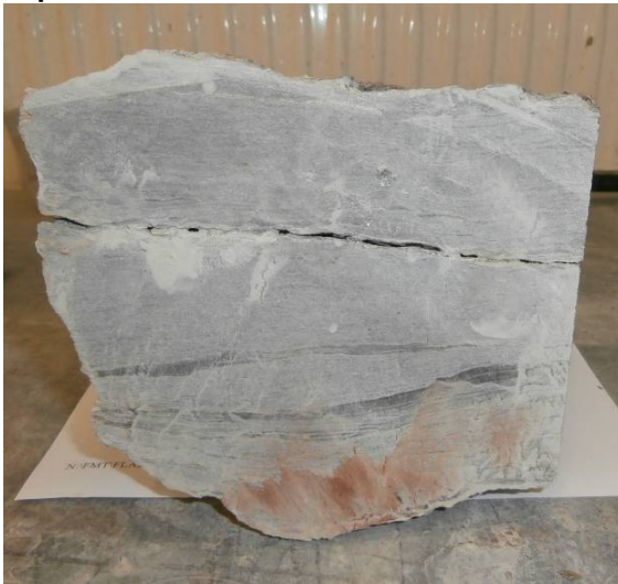
Sample 36/13s was split along a foliation plane before setting in grout
