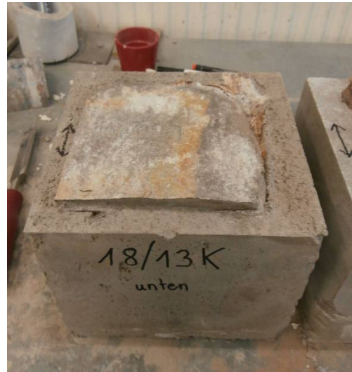
Sample half of the lower shear box after shearing (arrow marks the shear direction)
