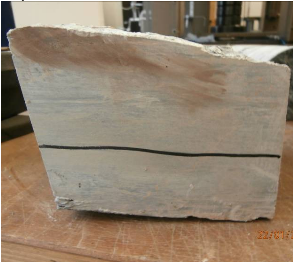
Sample before setting in grout (black line represents the estimated failure surface)
