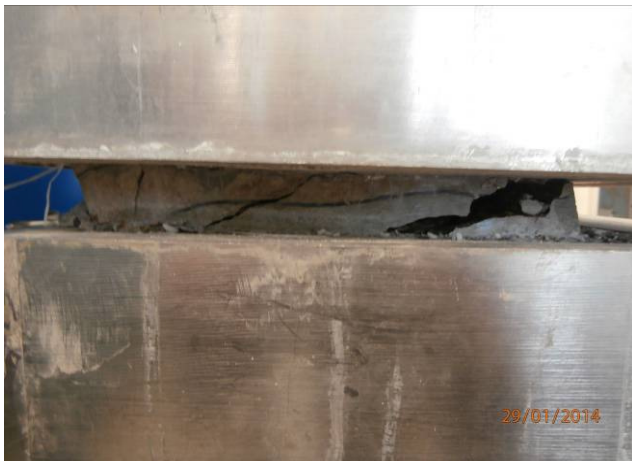
Sample 25/13s during shearing: The failure surface is not entirely located within the 2 cm gap between the shear boxes.
