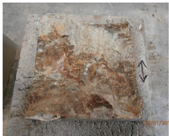
Sample half of the lower shear box after shearing (arrow marks the shear direction)
