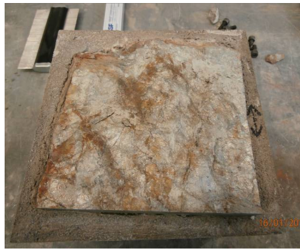
Sample half of the lower shear box after shearing (arrow marks the shear direction)
