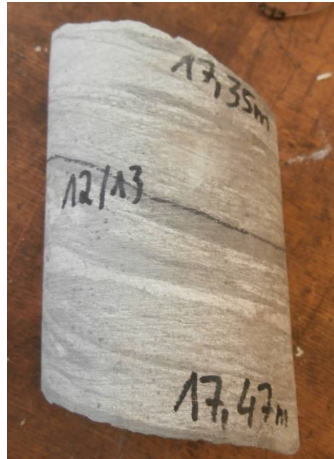
Core sample before setting in grout
