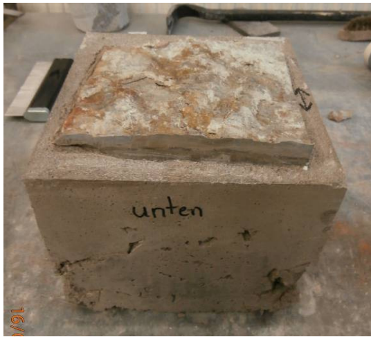
Sample half of the lower shear box after shearing (arrow marks the shear direction)
