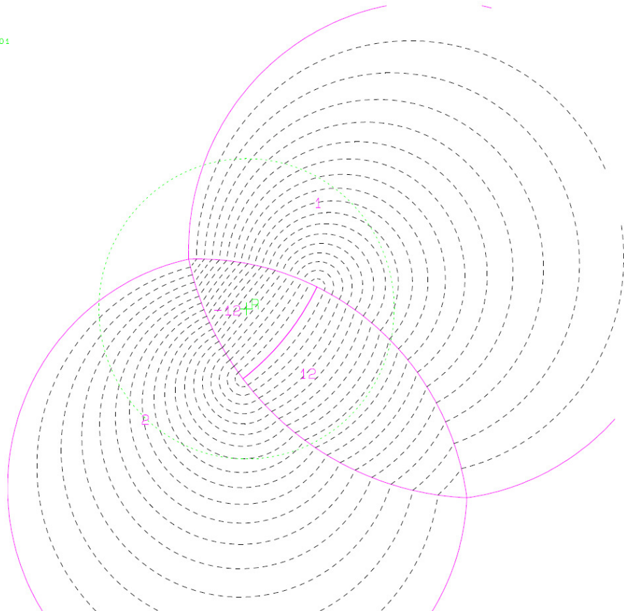
Contour plot of the friction angles for joint set j2 (= 1) and j5 (= 2) at outcrop 121. The green circle is the reference circle; R marks the resultant force vector.
