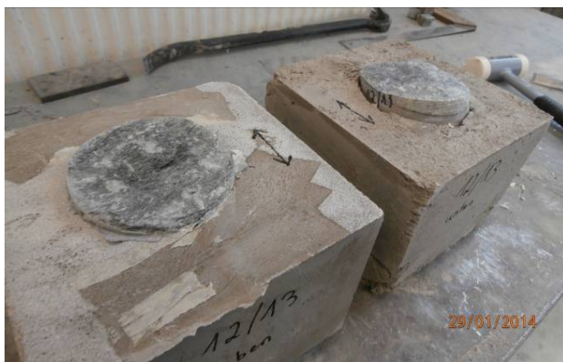
Upper and lower sample halves after shearing
