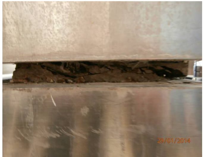
Sample 25/13s during shearing
