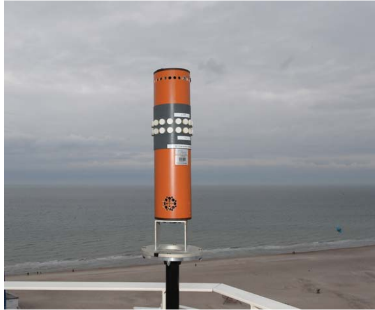
Figure 3.4: Antenna array for SIMO measurements
