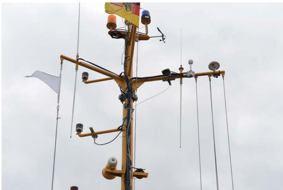
Figure 3.2: Ship mast with transmit and GPS antennas
