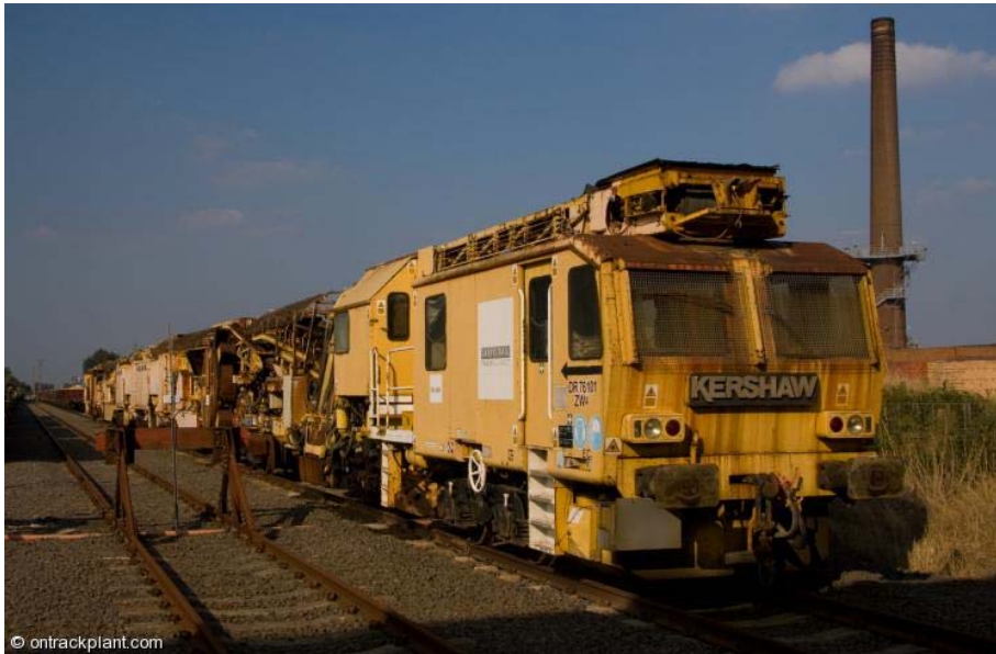
Picture 21: Ballast cleaning machine 33
