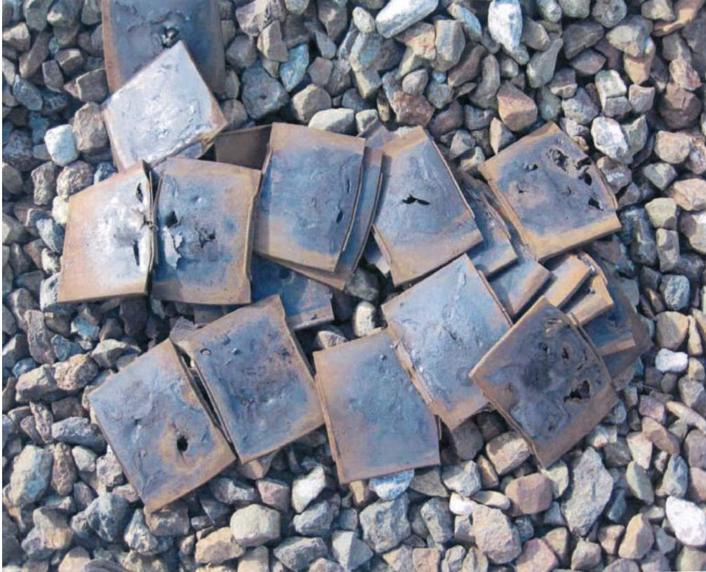
Picture 14: Rail pad wear
