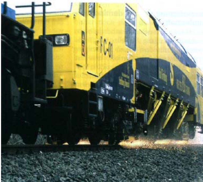
Picture 26: RC 01, Stahlberg Roensch 40 km/ h grinder 41
