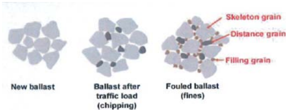
Picture 3: Ballast throughout the years 19
