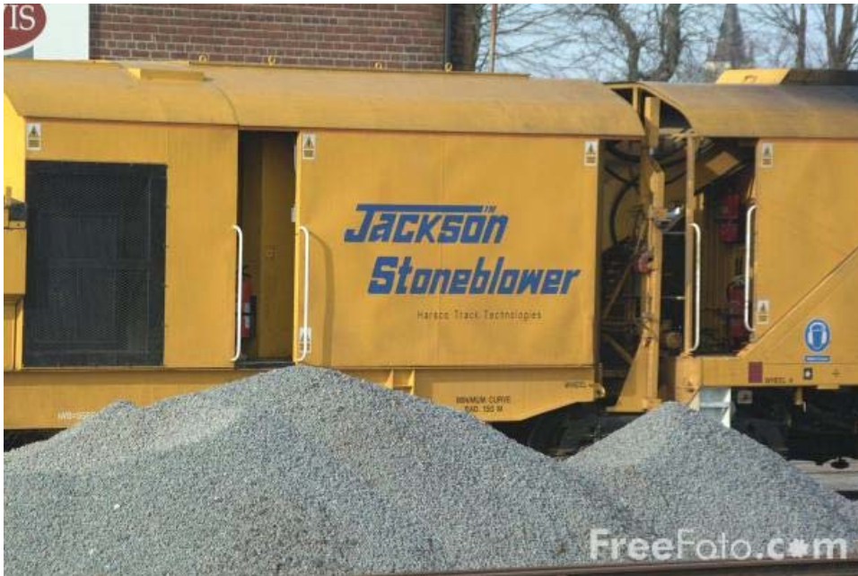
Picture 23: Ballast “stoneblower” 35
