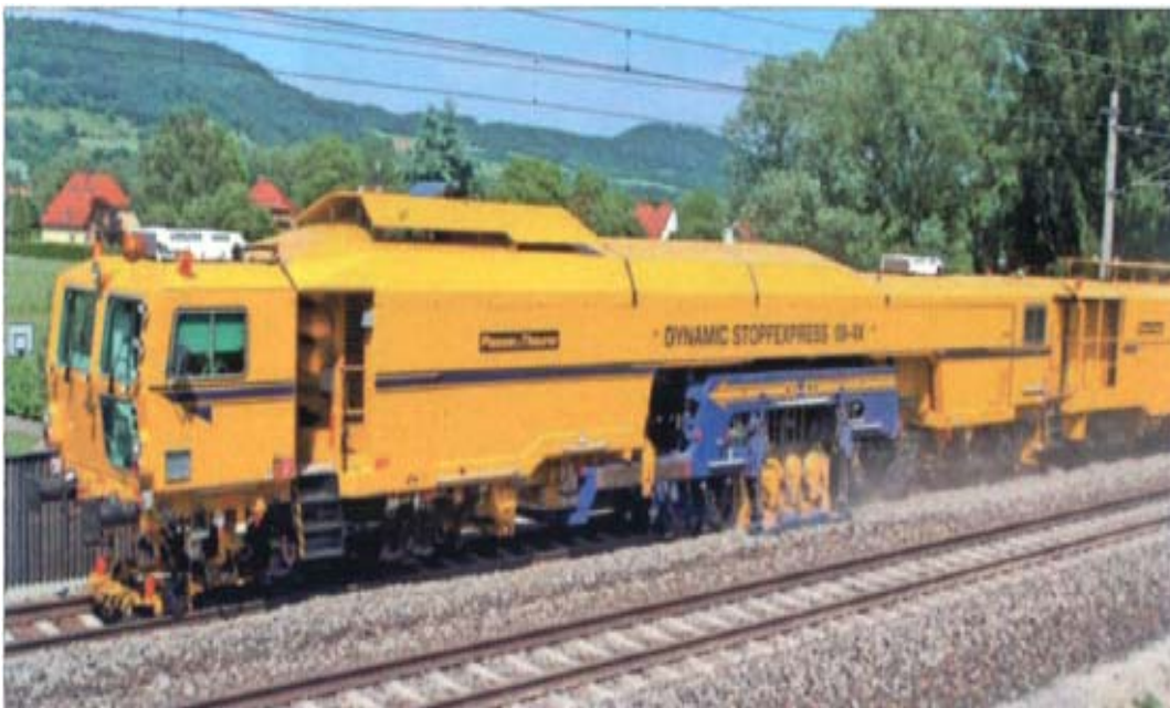
Picture 16: Continuous action four-sleeper machine with integrated track stabilization 28
