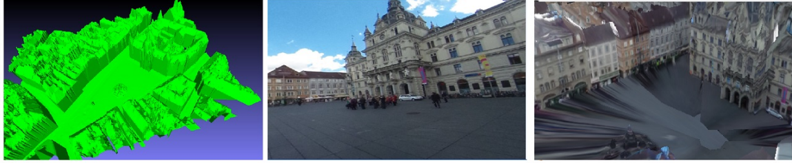
Figure 3.1: The system uses a solid geo-referenced model (left) and panorama images (middle) as input. Using projective texture mapping, both input data are combined to a virtual model of the environment (right).
