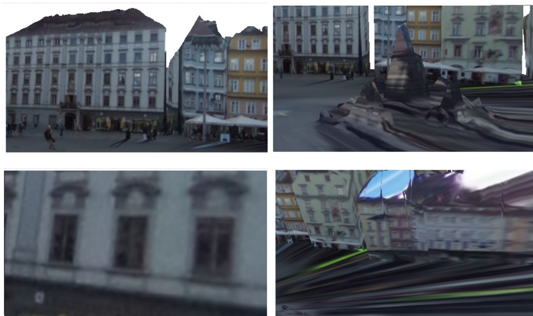
Figure 3.2: Our projection model works very well for facades of buildings (left, top). None of the used geo-referenced images is recorded close to a building, therefore, the image quality is reduced near buildings (left, bottom). Other issues are the low polygon count, which makes it hard to recognize the fountain (right, top) and problems caused by projective texture mapping (right, bottom).
