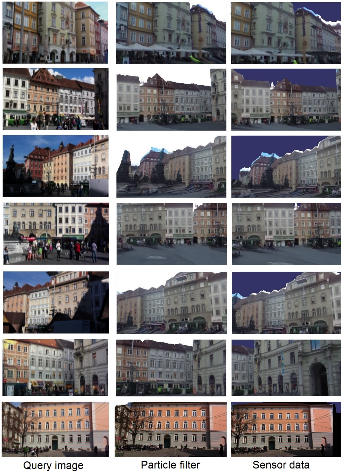
Figure 6.1: The input data for a pose query is an image from the smartphone (left) and sensor data from GPS and gyroscope. The device sensors are used as an initial guess (right). Our system provides an improvement of the initially guessed camera pose (middle). Note the robustness to issues such as occluding objects (first three rows) and shadows (fourth and fifth rows).
