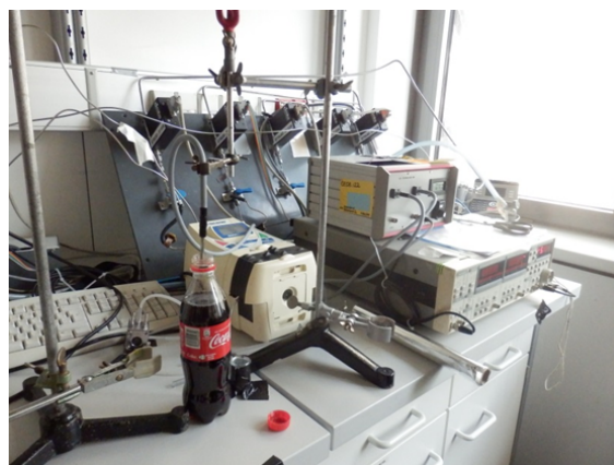
(b) Setup with lock-in, optic fibers and sensor foil
