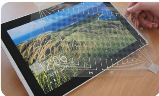
Figure 2.2.3. – Almost transparent PyzoFlex [48]
