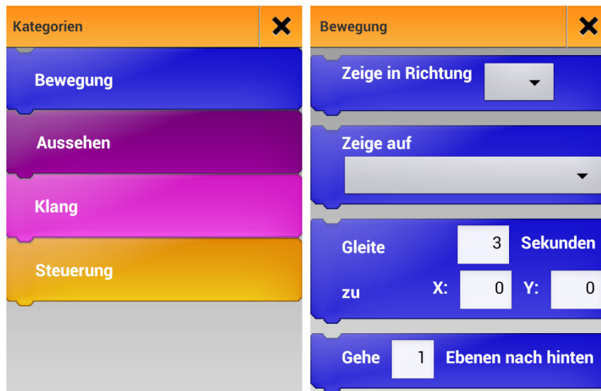
Figure 9.11: Catroid: add a new brick. Left: different categories of bricks. Right: bricks that are part of the “Motion” category.
