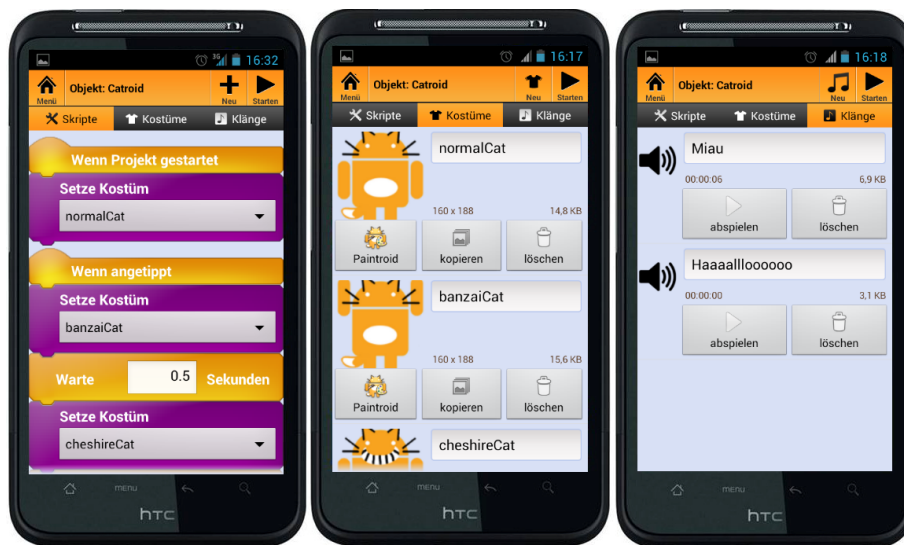
Figure 9.1: Catroid: three properties tabs of the object that is named “Catroid”. The image on the left shows the scripts tab containing several scripts. The image in the middle shows the costume tab with several costumes inserted. The image on the right demonstrates the sound tab.
