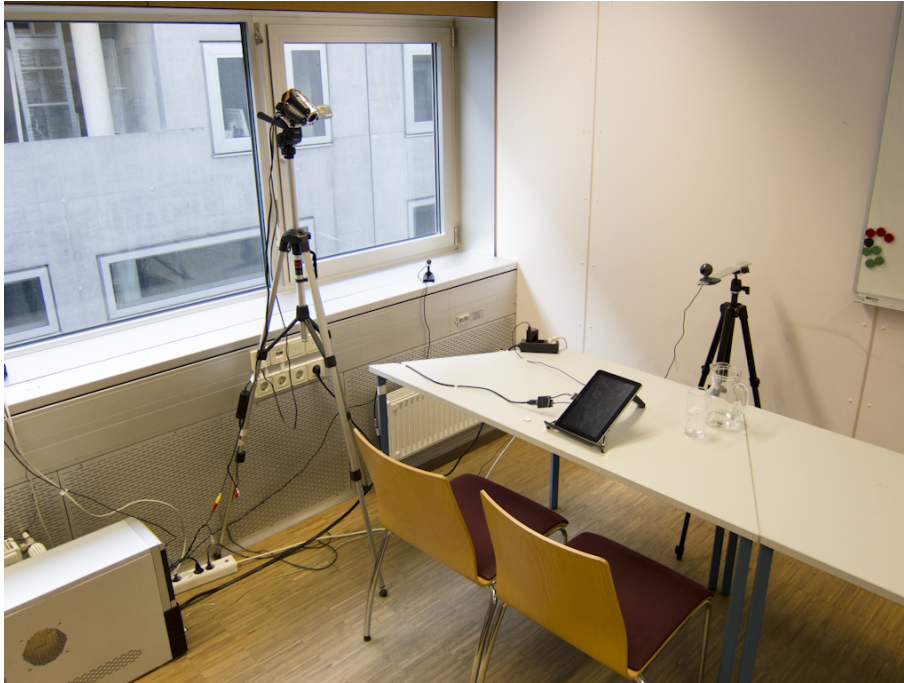
Figure 8.2: Usability laboratory especially built up for the test sessions. A web cam was mounted in front of the test users. A second camera was mounted on a tripod next to the users' seats. To ensure a consistently good view of the screen, the test device was fixed in a holder on the table.
