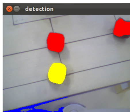
Figure 5.17: Final color detection, colored and automatically drawn in a camera image
