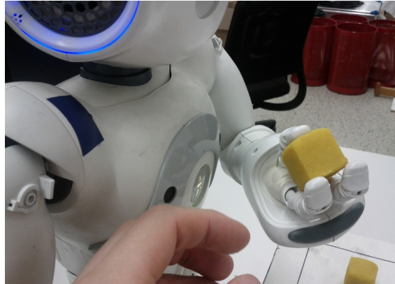
Figure 6.1: Pre-placement position of the hand, after the token has been recognized and the fingers have been closed, but before the hand moves to the target position.
