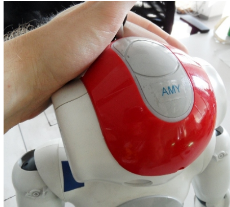
Figure 2.4: Touch sensors on the head module.
