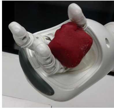
Figure 7.2: Unsafe grasp with two fingers
