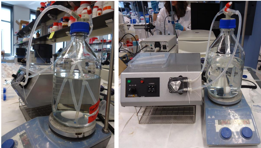
Figure 20: Setup for dynamic biofilm test on catheters.
