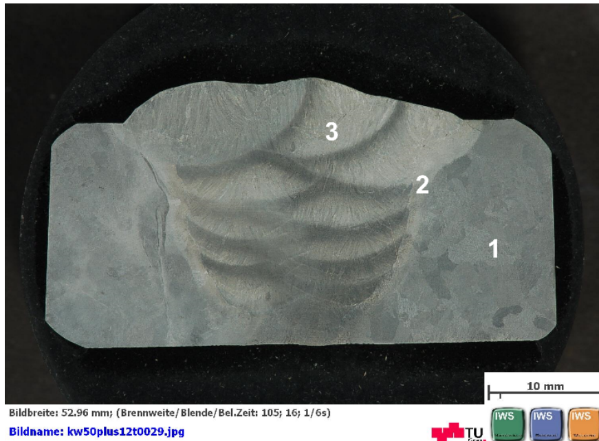
Figure 2.24.: Cross section of a weldment with marks of the different zones [2]
