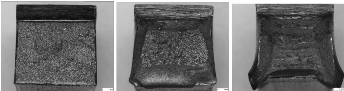
Figure 3.2.: Different types of the fracture [35]. Left) Brittle fracture. Center) Mixed fracture. Right) Tough fracture.
