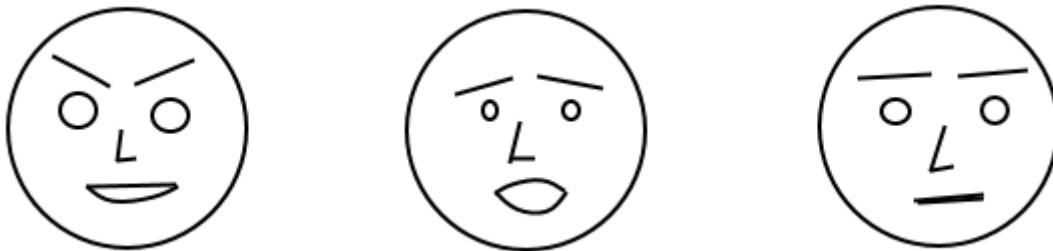
Figure 3.14: Three data records represented as Chernoff faces. The dimensions of the dataset are mapped to eyebrow slant, length of nose, and mouth openness. By observing changes in these facial attributes, the user can see how the values of the data records change in each dimension. [Diagram created by the author using paint.net [dotPDN LLC, 2015].]
