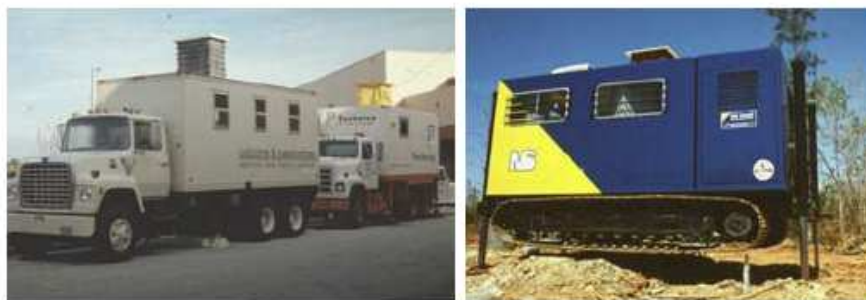
Figure 10: (a) Truck-Mounted and (b) Track-Mounted Cone Rigs (Mayne et al 2001)
