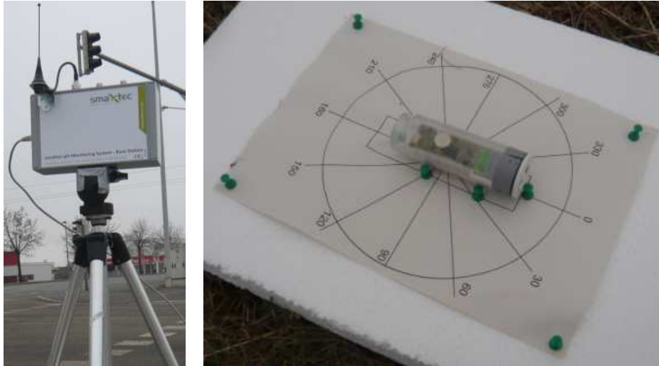
Figure 2.1: Test setup for open area test of smaXtec pH Bolus and Base Station. The left picture shows the Base Station with the connected rod antenna and the Ethernet cable. The right picture shows the smaXtec pH Bolus on a styrofoam plate with a compass rose for aligning the sensor.
