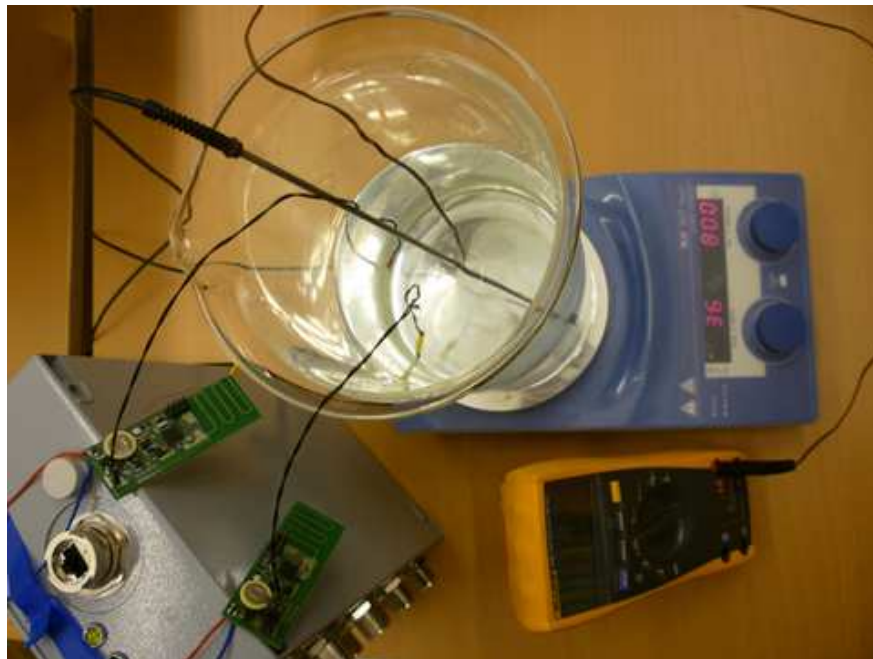
Figure 4.6: Arrangement for evaluation of temperature measurement with two Sensors (bottom left), Fluke 179 measuring temperature reference (bottom right), and a glass container on the RCT basic heating system (center).
