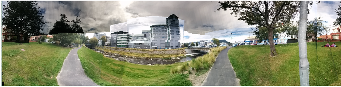
Figure 4.3: This panorama has been generated based on sensor tracking. Next to exposure time color artifacts, we can see that objects are not perfectly stitched together. For example the house and lamp look bent and the people on the right side are doubled.
