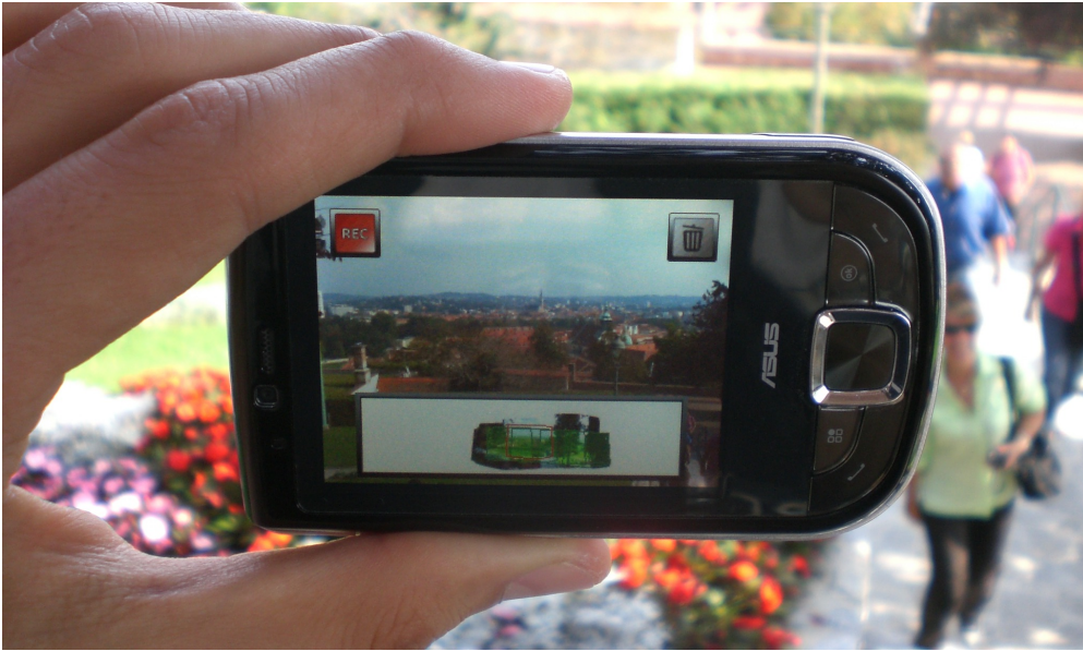
Figure 2.2: This photo shows the system of Wagner et al. (2010) in use, generating a panorama in real-time on a mobile phone.
