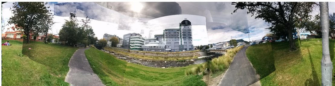
Figure 4.4: This panorama has been generated with PanoMT. We can again see exposure time and some other artifacts, but in general all objects are stitched together nicely compared to a sensor based panorama.
