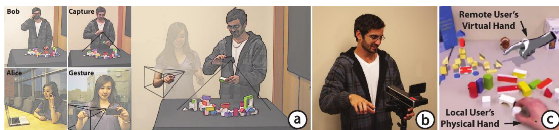
Figure 2.3: Sodhi et al. (2013) developed a mobile collaboration system called BeThere. The concept (a) shows two users, one capturing the shared environment and another gesturing. The environment and scene are captured with depth cameras (b) and the virtual hand is integrated into the camera image of the workspace (c).
