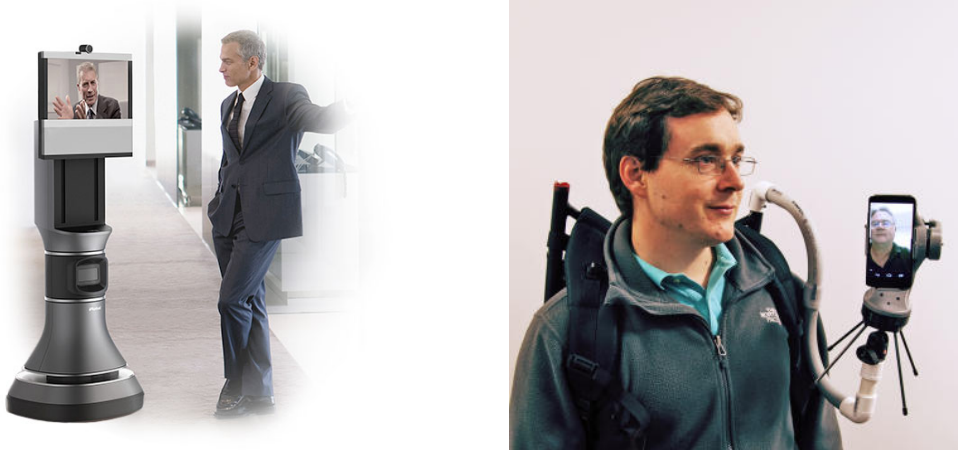
(a) The iRobot Ava ® 500 video collaboration robot 6 . This is a mobile telepresence robot targetting the business market. (b) Polly, the parrot smartphone robot in use by Kratz et al. (2014). The remote user controls the view.
