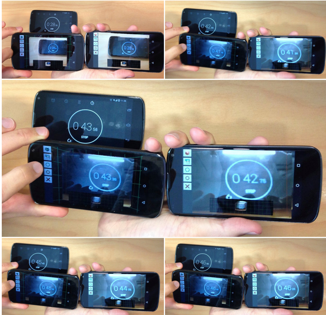
Figure 5.15: These photos are used for end-to-end latency measurement. The upper left phone shows a running timer, while the lower phones are running the telepresence application. The left of these two phones is the local phone and the right one the remote phone.
