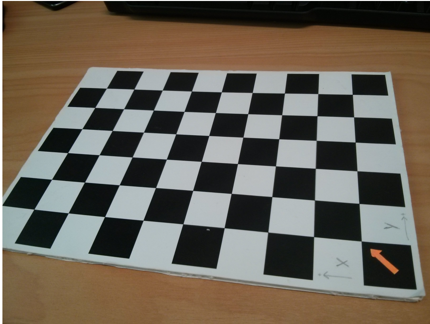
Figure 4.1: A checkerboard pattern with 9 \times 6 inner corners has been used to calibrate the cameras with the OpenCV camera calibration application. This is one of the calibration photos of a Nexus 4 smartphone.
