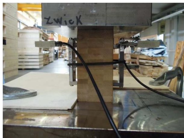
Figure 20: Test setup for compression tests perpendicular to the grain
