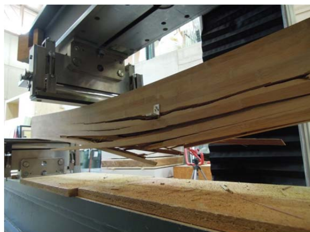
Figure 27: Typical failure mode due to bending (left) B-A1 (FW); (right): B-A2 (EW)
