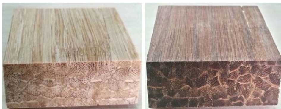
Figure 14: Cross section of bamboo scrimber: (left) natural (right) carbonized (Yu, et al., 2015)
