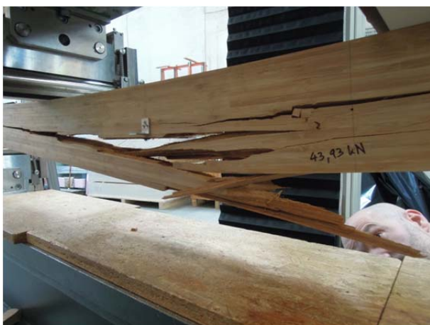
Figure 27: Typical failure mode due to bending (left) B-A1 (FW); (right): B-A2 (EW)
