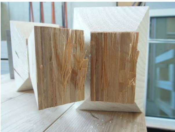
Figure 28: Typical failure mode due to tension perpendicular to the grain (left) T90-G1 (EW); (right) T90-G2 (FW)
