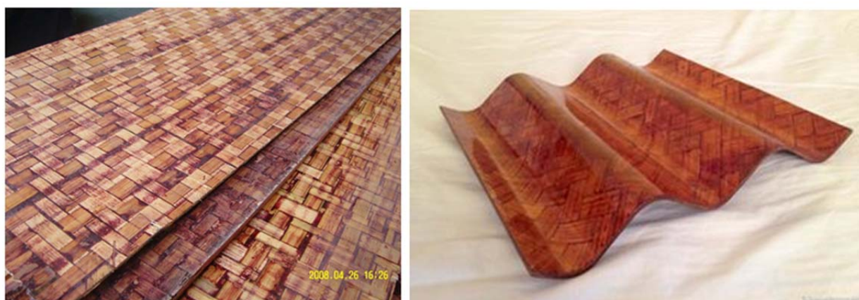
Figure 16: (left) Bamboo mat board (Foshan Ying plus earnings Wood Co, 2013); (right) roof sheet made from bamboo mats (Schröder, 2014)
