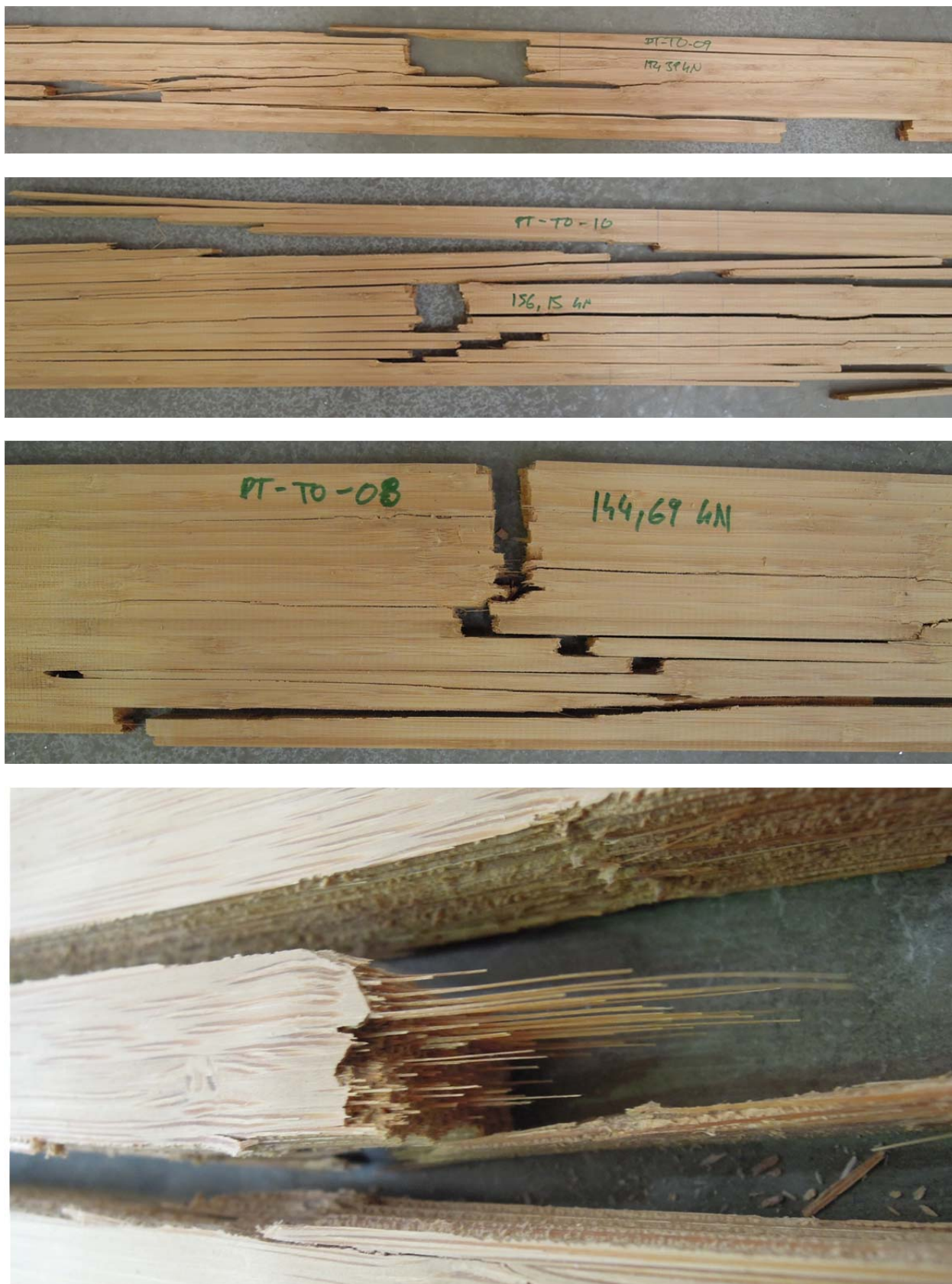
Figure 30: Typical failure pattern due to tension; detail of torn out fibres
