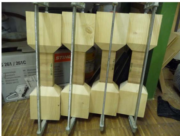
Figure 22: Manufacturing process of the samples for the T90-tests
