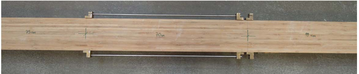
Figure 25: Specimen with mounted rods as base line for measuring the local deformation
